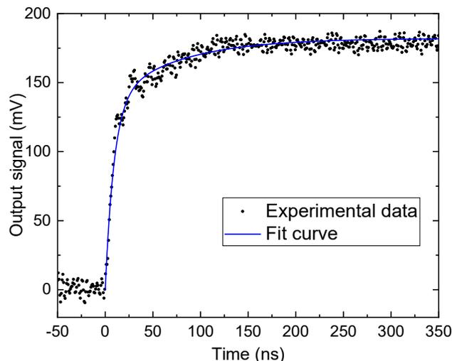
Fig. 1. Example of output signal of the charge amplifier generated by the photoelectric absorption of a 59 keV photon ( $^{241}\text{Am}$ ) and acquired with the custom designed ultra-low noise fast readout electronics. The electron and hole signal components can be discriminated and analyzed with high resolution.
