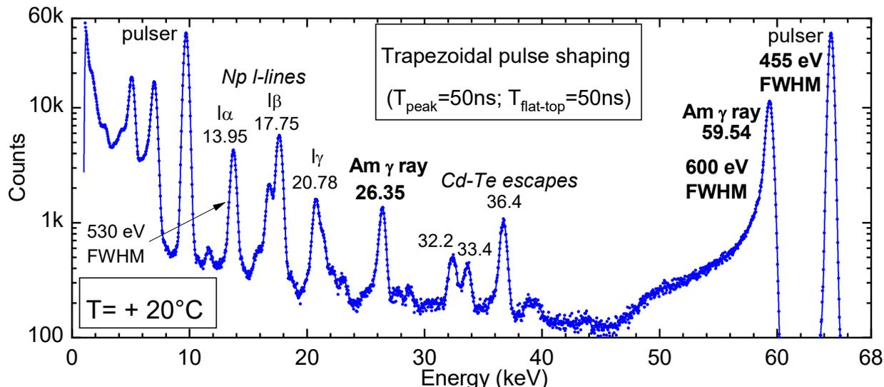
Fig. 2.  $^{241}\text{Am}$  spectrum acquired with the CdTe detector and SIRIO preamplifier at  $+20^\circ\text{C}$ , 700 V of bias voltage and 50 ns of pulse shaping peaking time.
