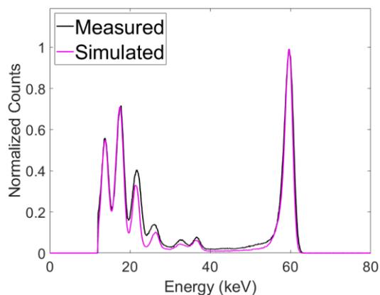
Figure 3. Comparison between experimental and simulated energy spectra of  $^{241}\text{Am}$  nuclear source.
