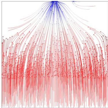
Figure 2. Example of interaction positions and electrons trajectories in a hemispheric detector.
