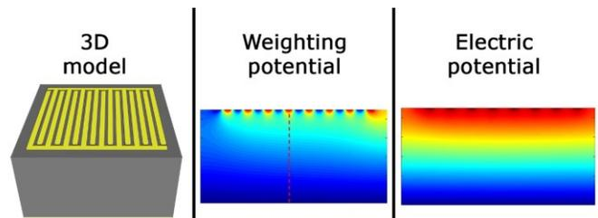
Figure 1. Example of coplanar detector (left) and related weighting (centre) and electric potential (right).
