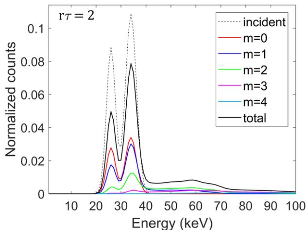
Figure 2. Simulated spectrum distorted by peak pileup effect at high flux ( $r\tau = 2$ ). The dashed line represents the undistorted spectrum. Peak pileup spectra up to  $m = 4$  are showed as colored curves.
