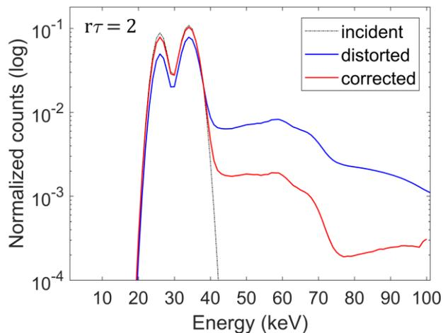
Figure 3. Correction of the distorted spectrum at high flux ( $r\tau = 2$ ) showed in Figure 2. The dashed line represents the undistorted spectrum.
