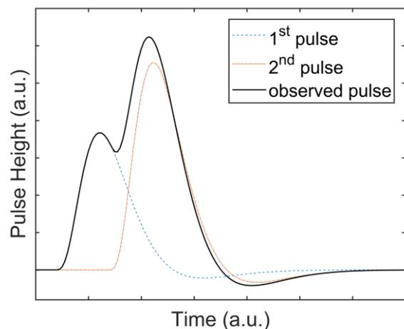
Figure 1. Example of peak pileup effect in the case of two bipolar pulses.
